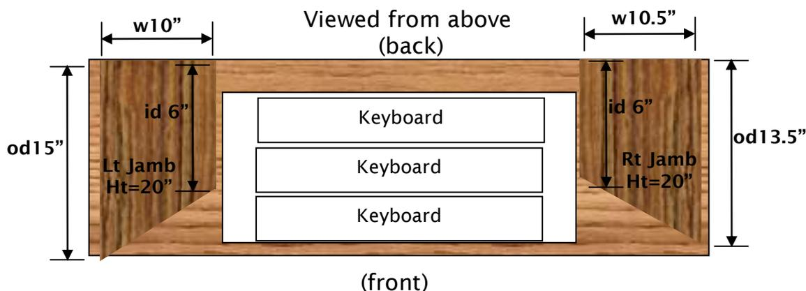
The measurements in the diagram above show the height (Ht), outside depth (od), inside depth (id), and width (w) of the stop jamba. They are not quite identical because, when a 30-note pedalboard is used, the keyboard stack is not exactly central in console.
